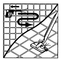
8. Turn Chemical off. Pressure clean by rinsing surfaces at high pressure.
